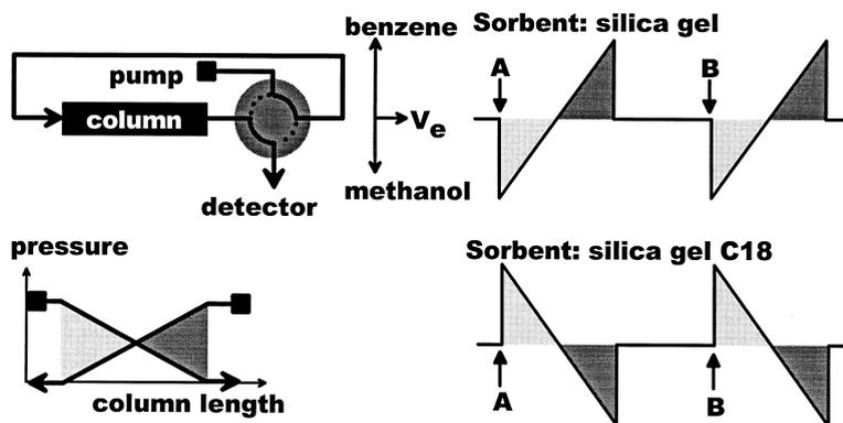
**Figure 3.** The shape of zones (schematically) generated by column backflushing. Symbols as in Fig. 2.
