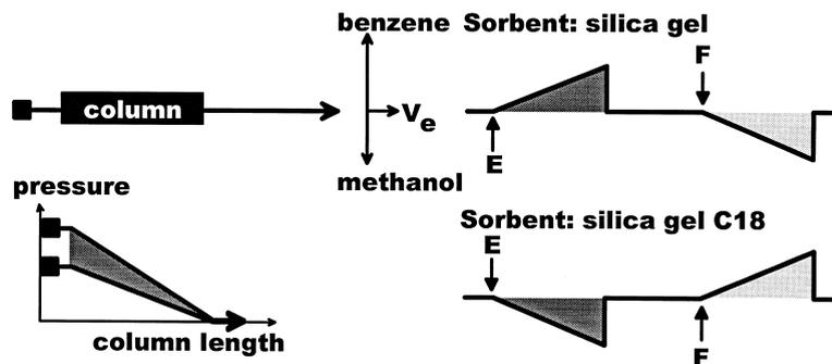
**Figure 4.** The shape of zones (schematically) generated by sudden change in flow rate. E = increase in flow velocity; F = decrease in flow velocity. Symbols as in Fig. 2.
