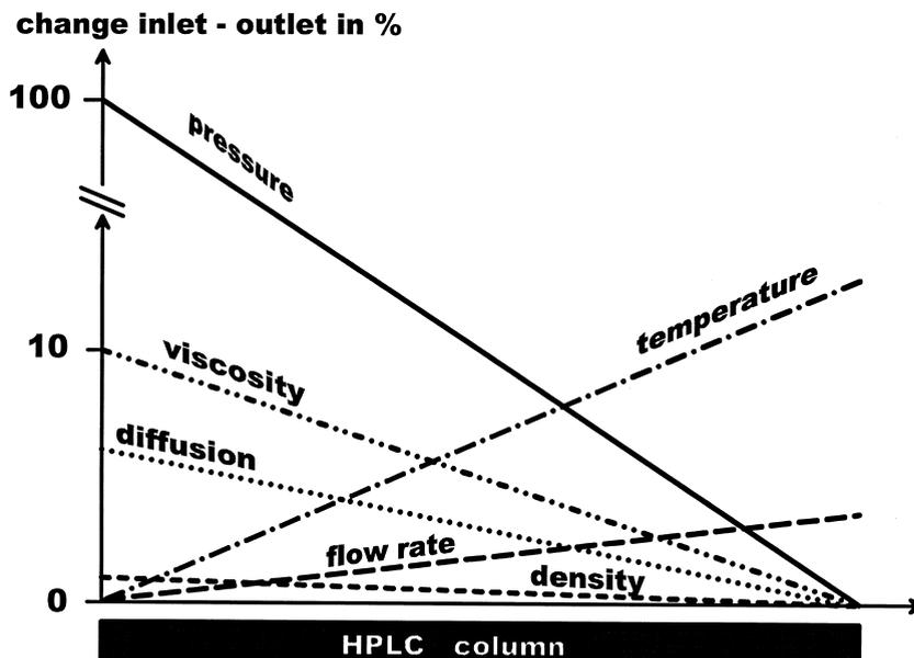
**Figure 1.** Schematic representation of longitudinal profile of pressure, flow velocity, viscosity, density, temperature, and diffusion within a homogeneously packed non-thermostated HPLC column (Constructed according to data from refs. 2, 3, and 5).
