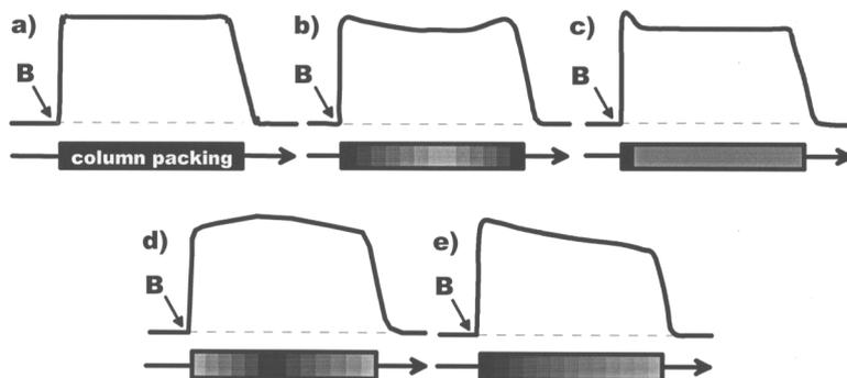
**Figure 8.** Dependence of zone shape on column packing density. Smaller packing density of sorbent in column = light gray area, larger packing density = dark gray area.
