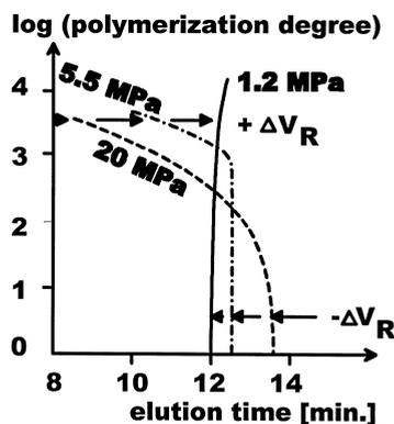
**Figure 7.** Dependence of elution behaviour of polystyrenes on pressure. Eluent: chloroform / tetrachloromethane, 4.5/95.5, v/v. Column packing: Porous glass. Figure constructed according to data.<sup>37</sup>
