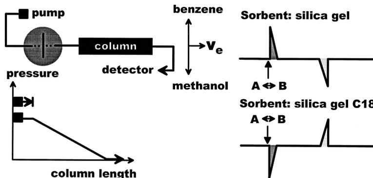
**Figure 5.** The shape of zones (schematically) generated by short interruption of flow applying a valve situated before column. Symbols as in Fig. 2. For detail explanation see ref. 25.
