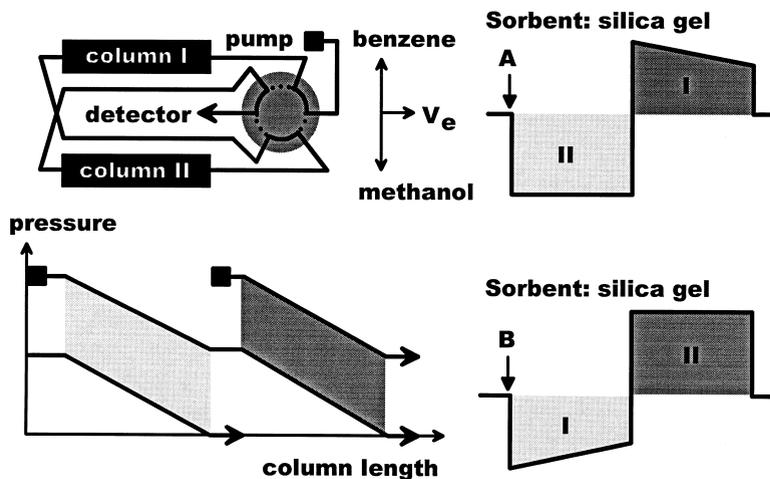
**Figure 6.** The shape of zones (schematically) generated by alternate recycling. Symbols as in Fig. 2.
